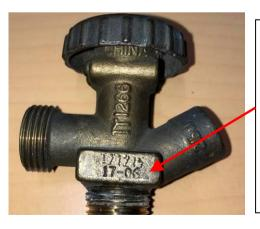
**STEP 3** Carefully examine the side of the valve body. The manufacture date (YY-MM) can be located at the base of the valve on the flat. If this is **17-06** or **17-12** then the cylinder is to be recalled.
