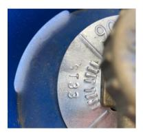
**STEP 1** The NEXT TEST code is a combination of letters and two numbers. If the test code consists of numbers 33 or 34 the valve manufacture needs to be checked. GO TO STEP 2
